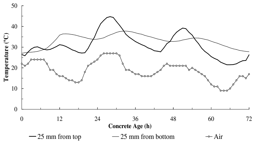
Figure 260. Measured concrete and air temperatures for North Carolina, Slab 4.
