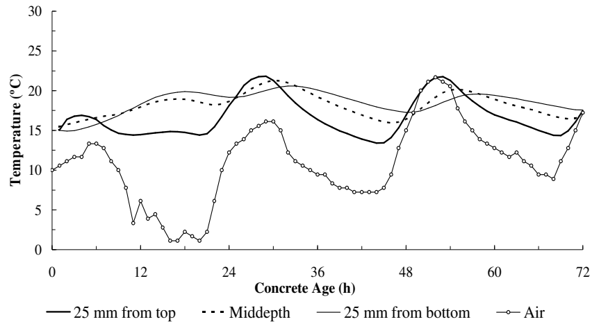
Figure 232. Measured concrete and air temperatures for Minnesota, Slab 2.
