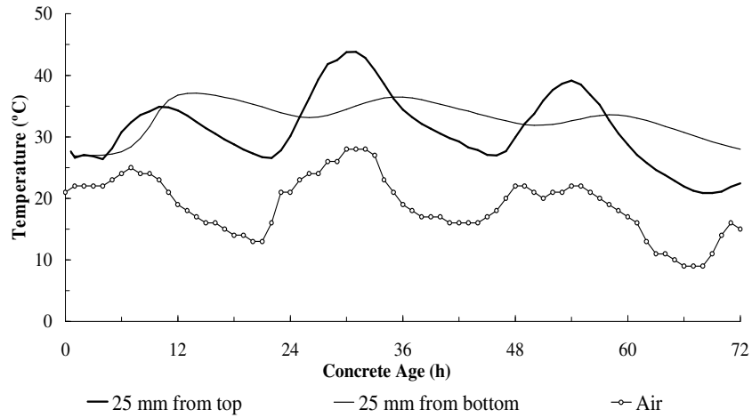
Figure 228. Measured concrete and air temperatures for North Carolina, Slab 3.
