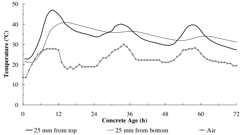
Figure 220. Measured concrete and air temperatures for Lufkin, TX, Slab 3.
