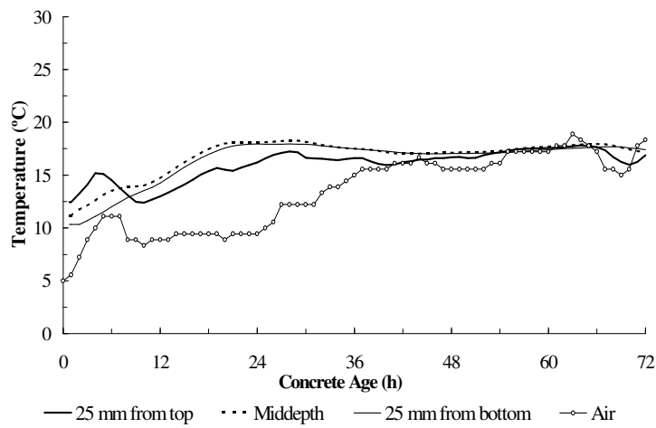
Figure 200. Measured concrete and air temperatures for Minnesota, Slab 4.
