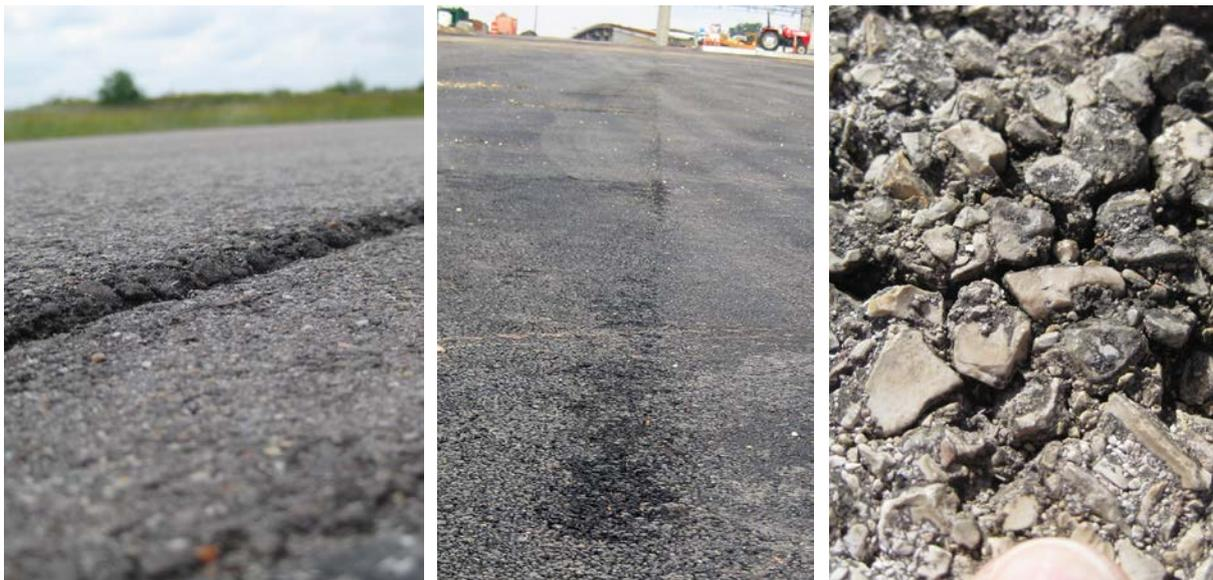
Figure 1 – Poor joint construction (a,b) and deteriorated asphalt material (c)
