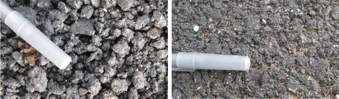
Figure 2 – Segregated asphalt can lead to coarse texture (a) within a meter of fine texture (b)
